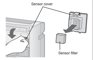
Remove the Sensor cover, and remove the dust on the Sensor filter.
